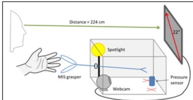
Figure 2 - The experimental setup consisting of a non-transparent box with a lid, a simple laparoscopic grasper, a 22 inch monitor with horizontal resolution 800 lines, a web cam, a force sensor, a spotlight and tape to mark the position of the force sensor.
